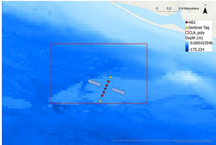
Figure 10: Deployment location for the line of acoustic receivers and sentinel tags used in the range test.
