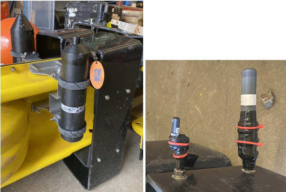
Figure 2: LEFT: Receiver mounting system. The 170/180 kHz HR2 receiver is mounted on the starboard side with the 69 kHz VR2W receiver on the port side. RIGHT: Mounting system for 170/180 kHz tag (left) and 69 kHz PPM tag (right). The tags are mounted to the top of the tail fin.
