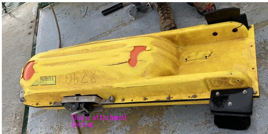
Figure 36: Wear on one side of the SUB at mooring 3. The photograph is oriented in the same sense of the deployed SUB, with the lower part of the image corresponding to the lower part of the SUB which is tethered by a chain to a bottom weight. Photograph by Louise McGarry, FORCE.
