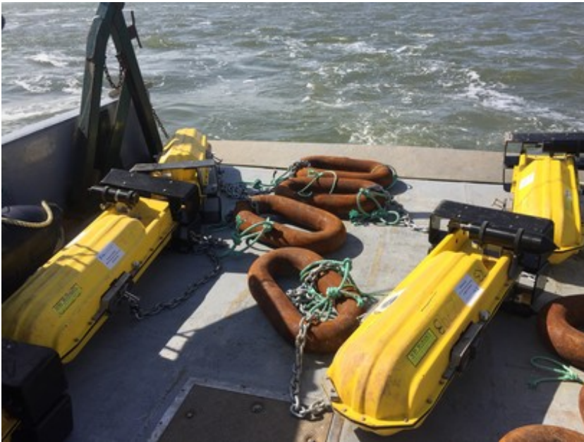
Figure 1: SUBS floats, loaded with range test equipment. A large, 500 lb chain link serves as the anchor and it is attached to the SUBS by a 2 m chain link that also serves as a riser cable. (Photo: Charles Bangley.)
