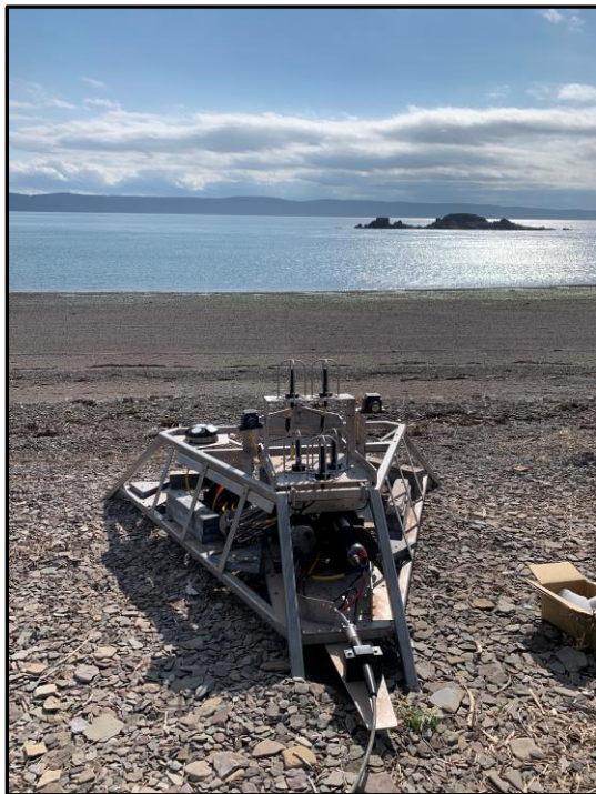
Figure 13: The cabled subsea platform developed for the VITALITY project just prior to deployment in the intertidal zone.
